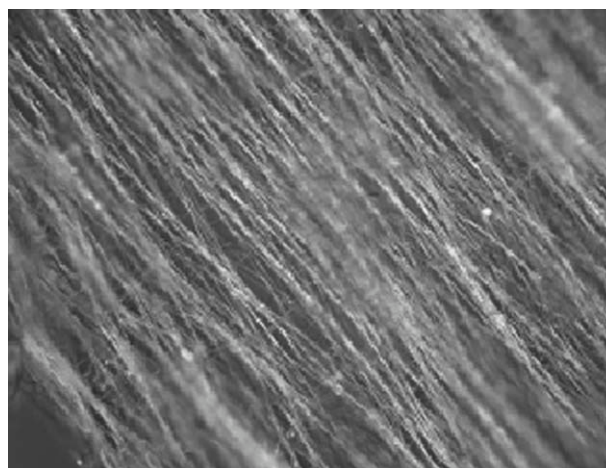
Figure 4 Sample 27-6-24 (27% solids, 6% GLY, 24°C, 30 min) at 400× using cross-polarizing filters detailing birefringence of fibers.
